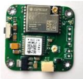
DroneBeacon Db121pcb RemoteID Broadcast Module
